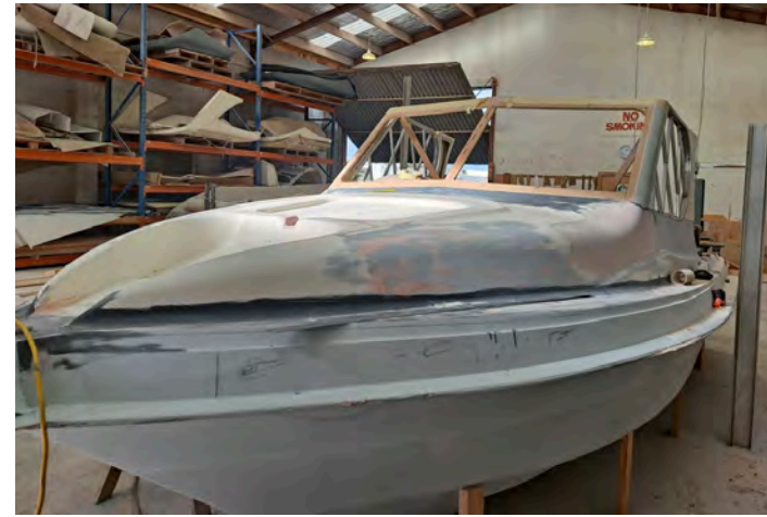
To make sure they had the lines right, a mockup of the hardtop was made before production began.
