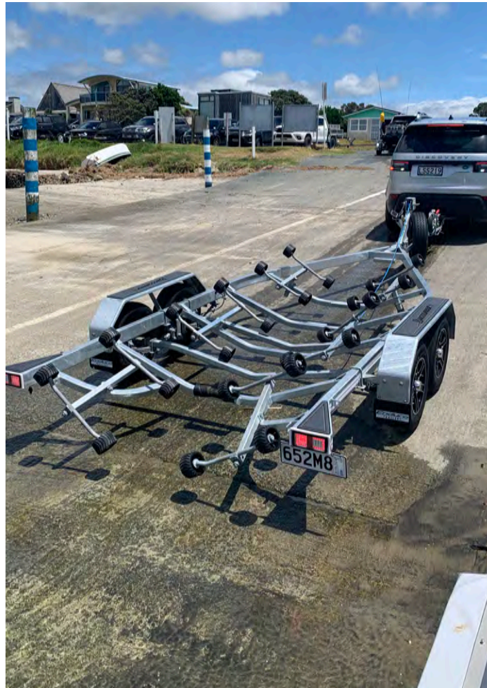
The Enduro multi-roller trailer is braked using an override system.
