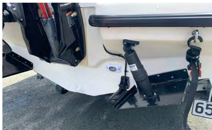
Trim tab bases are recessed into the transom.
