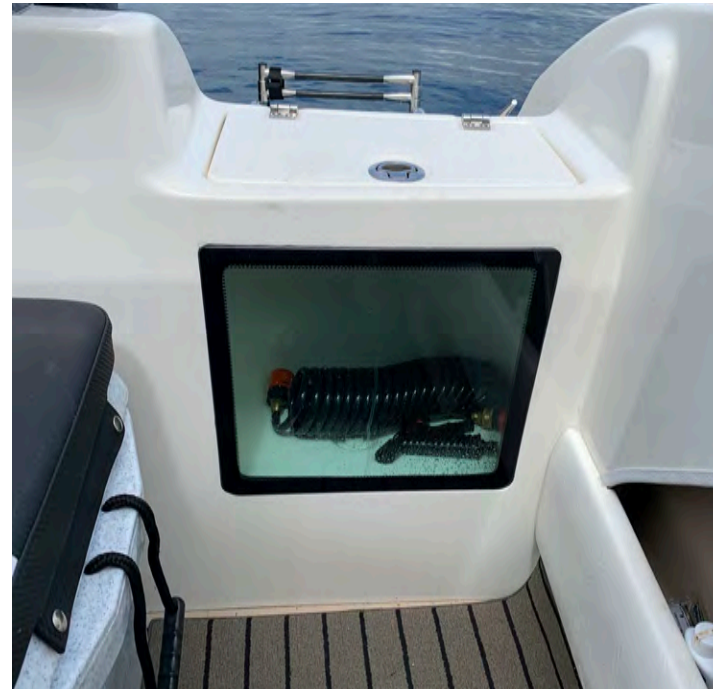
The livebait tank aerator and the washdown hose run off the same pump.
