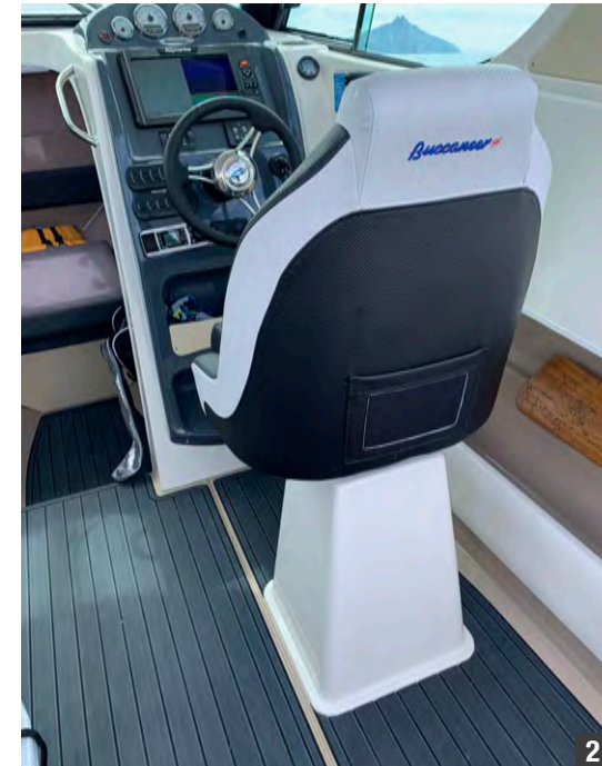
1) Buccaneer's bespoke rod holders. 2) Pedestal seat bases have minimal intrusion into the cockpit space. 3) There is plenty of room to overnight on the full-length bunks.
