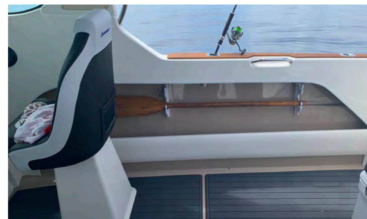
Full-length cockpit side shelves are fitted with holders for rods, gaffs, paddles and the like.
