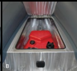
PICTURE A OPTIONAL ALUMINUM JOCKEY SEAT WITH COMPARTMENT FOR FUEL TANK
